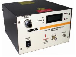
Spellman's Bertan brand of 230 Series high voltage power supplies provide regulated high voltage outputs from 1 to 30kV. The low noise, linear topology employed results in extremely low output ripple specifications. These 12 to 15 watt units are inherently reversible by design, providing either positive or negative output polarity. The 230 Series is fully arc and short circuit protected. Excellent regulation specifications are featured along with outstanding stability performance.
